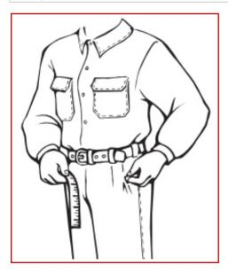
Size your body belt using a tape measure to obtain the correct D-to-D (D-ring to D-ring) size, measure around the back from hipbone to hipbone and then add 2" (51 mm)
